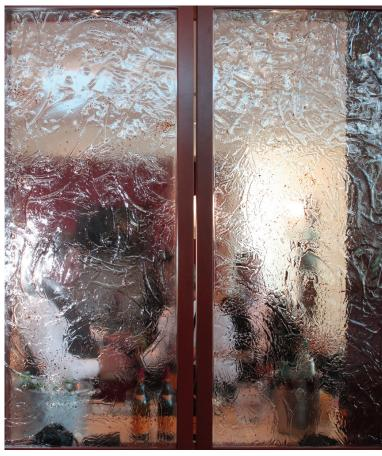
Texture: MD102 Stucco 1/4" Clear Tempered Kiln-Fired Glass with Dichroic Glass on Smooth Side
